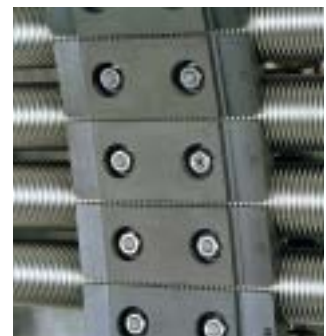
Fusion experiment TEXTOR, JÜLICH RESEARCH CENTRE: The temperature and vacuum resistant SINTIMID PUR HT was used to produce retaining clips for current coils used to generate magnetic fields.
