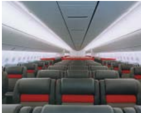
Luminaire covers used in a BOEING 777. The transparent material TECANAT PC is self-extinguishing and offers good welding capability.
